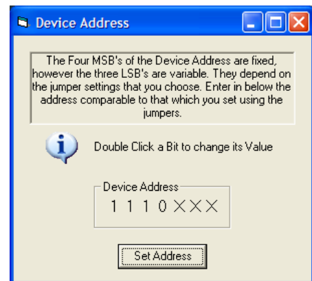
Figure 3. I 2 C Address Selection
